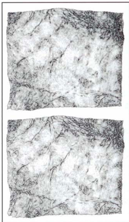
FIGURE 2 Similarity Attribute on a Mapped Horizon Before (Top) And After (Bottom) Fault Enhancement Filtering
